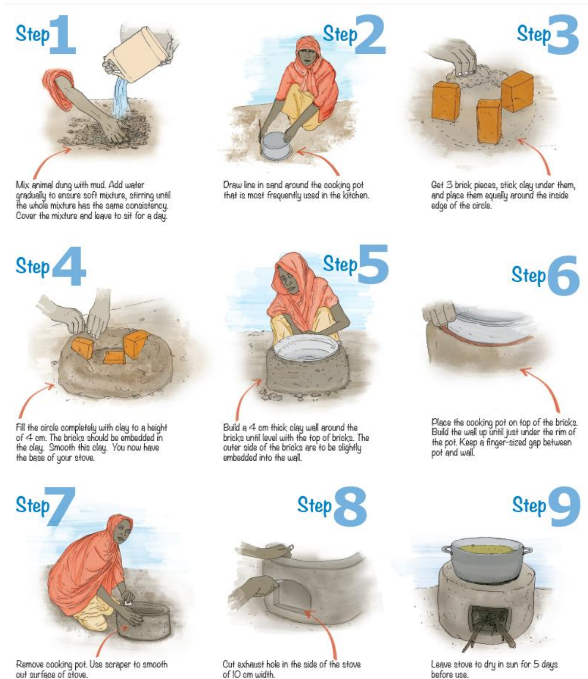
Figure 2: How to make Fuel-Efficient Stoves – step-by-step (Source: WFP, 2015 )
